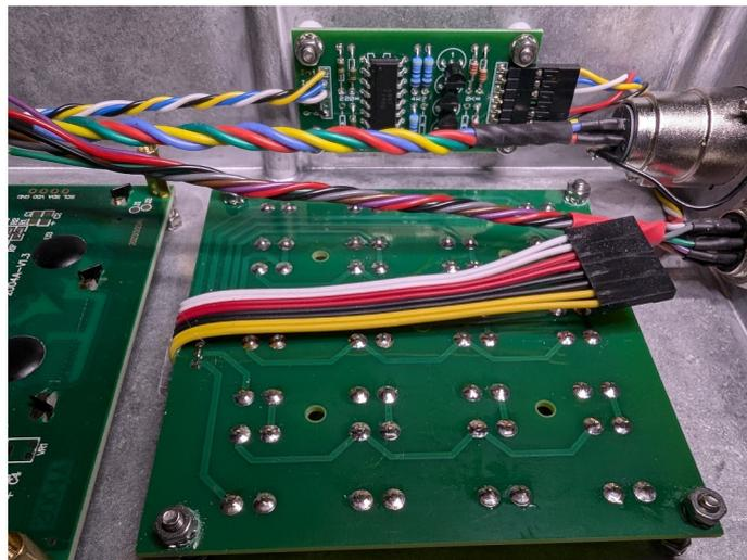
To adjust the height of the keypad it helps if it's a bit tight on the screws (it usually is).
