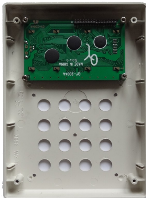
Fig 3 – Case internals with LCD fitted.
