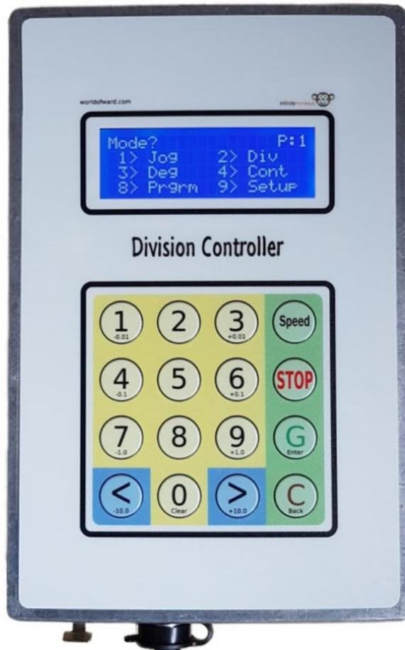
This document explains how to put together the hardware to create a division controller. It covers machining the case, wiring the various sockets and modifications to the stepper driver to enable it to fit.
