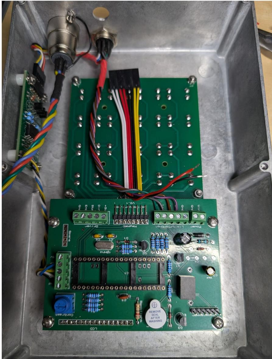
Next we can fit the power connector – make sure the negative connector is pointing down to prevent it fouling on the stepper driver.
