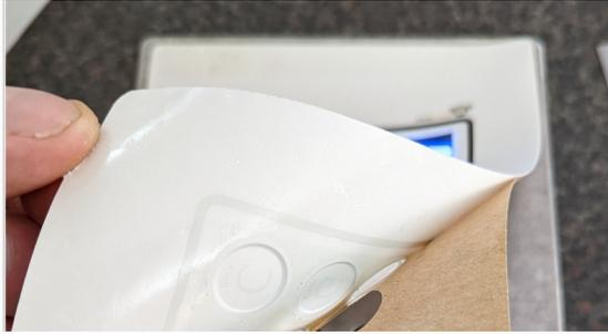
Hinge the overlay back and peel off the backing.
