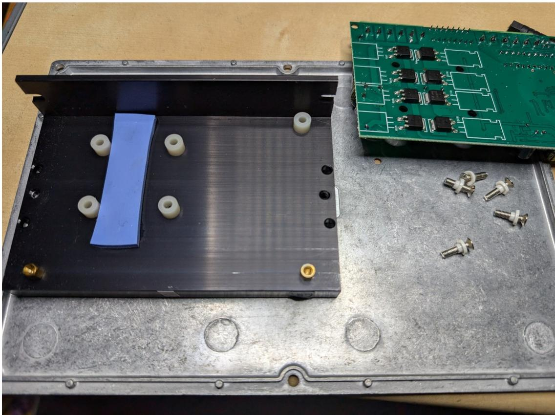
In the case of the thermal pad version we'll put the pad over the surface mount transistors making sure it covers them.
