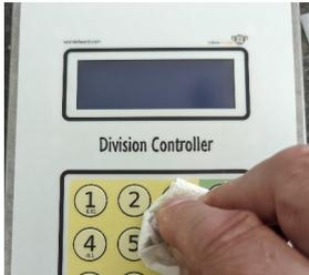
Use a soft cloth and a moderate amount of pressure rub over the overlay to stick it down to the case. Start from the middle and work out to express any air.
