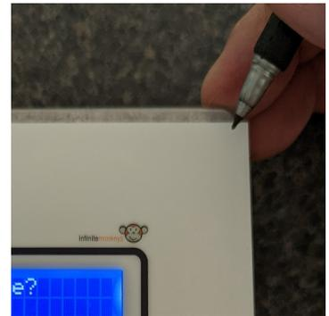
I recommend a straight edge and craft knife, taking several light cuts rather than one cut (which can pull the overlay over resulting in the cut drifting).
